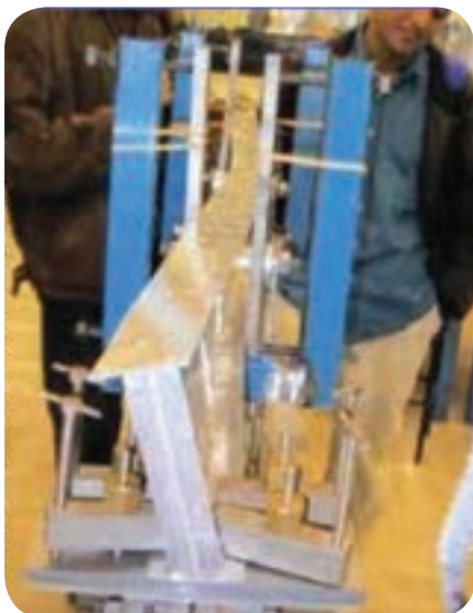
Figure 8: Lateral torsional buckling
