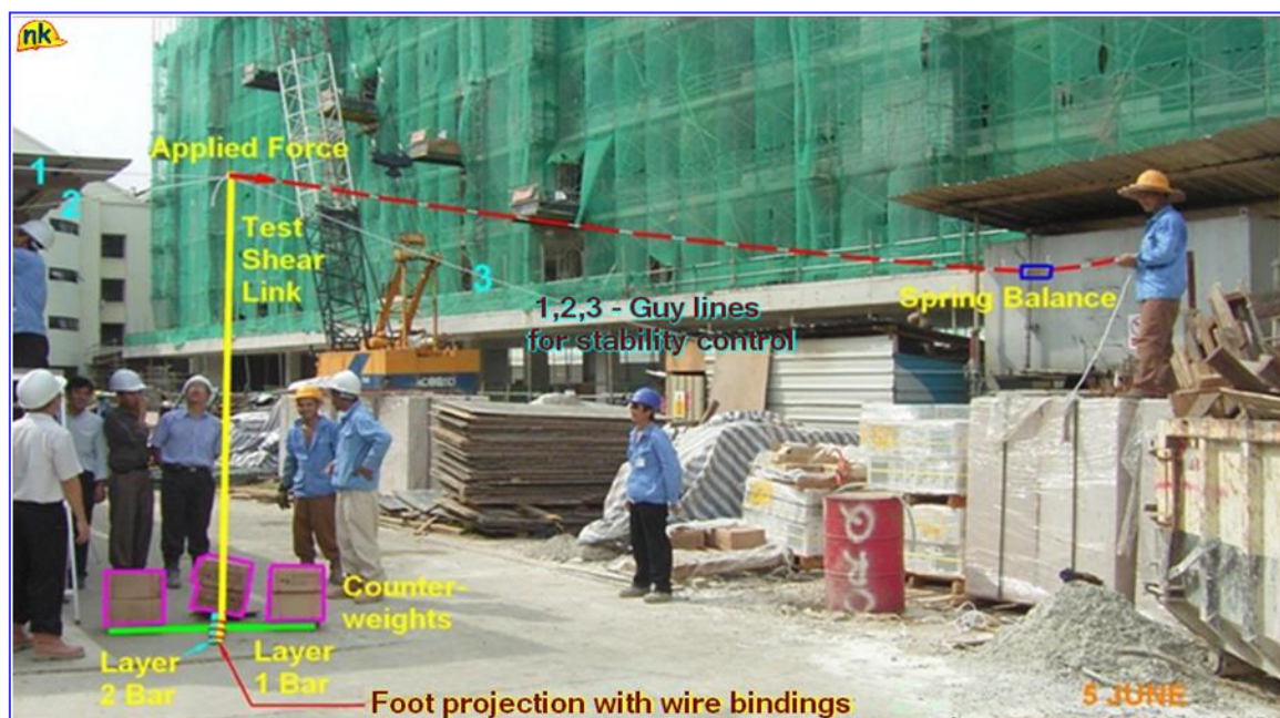
Fig. 17. Author's field test for rotational capacity
