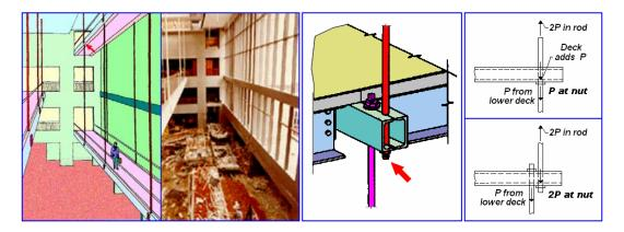
Fig. 1 (Left pair) Hyatt Regency Walkway, Before and After the Collapse; (Middle) Nut at Upper Walkway; (Right) Static Analysis of Single versus Double Hanger Rods.
