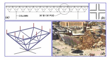
Fig. 3 Hartford Civic Center Arena: (a) Schematic Section; (b) Cruciform Section Used; (c) 30' by 30' pod; (d) Collapse Scene.
