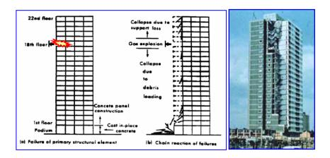
Fig. 2 Ronan Point: Schematic of Collapse, and Photograph.
