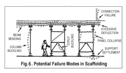
checked and approved, is a very common cause of the base sinking under concrete placement or other heavy loading.
