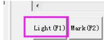
Change X/Y value in the software or move the moveable platform to adjust the red light position.
