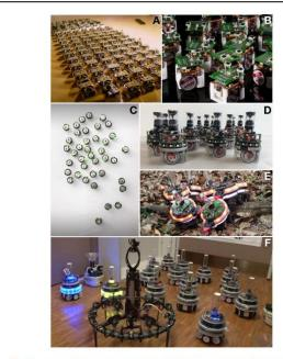
Fig. 2. Some of the robots largely used in swarm robotics research: (a) Jasmine [35] (photo: WikiMedia Commons); (b) alice [36] (photo courtesy of Simon Garnier); (c) kilobots [30] (photo courtesy of Massimo Berruti); (d) e-pucks [37]; (e) swarm-bots [26]; and (f) swarmanoid [29].
