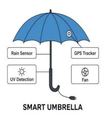
Rain Prediction Module – A combination of a humidity and temperature sensor (DHT22) and an external Weather API helps to forecast rainfall in the next 5–10 minutes. If rainfall is predicted, the umbrella immediately sends an alert to the user through the mobile application or an inbuilt notification system (buzzer/LED).
