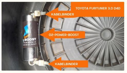
The air flow typically flows from bottom to top into the air filter, with the booster positioned in the air flow before the filter.
