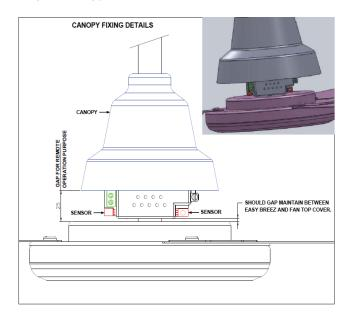
Note: Leave a clearance of 25mm (1inch) between top cover of the fan and lower canopy as show above for best remote signal reception
