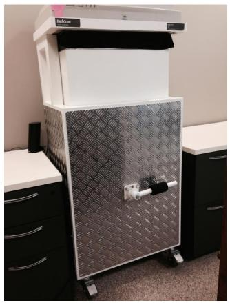
Figure 1. This workstation is for capturing high resolution specimen images. Here, it's shown closed. By pulling the lever to the left, a space just above the silver part of the cart will open. Pulling the lever to the right will bring the specimen close to the scanner (shown at the top, upside down) for image capture.
