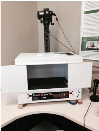
Figure 2. This workstation is for capturing lowerresolution specimen images. Here, it's shown open and with the lights off. By opening the doors at the front, a specimen can be placed inside. Closing the doors and controlling the camera (mounted above the box) using an attached computer facilitates image capture.
