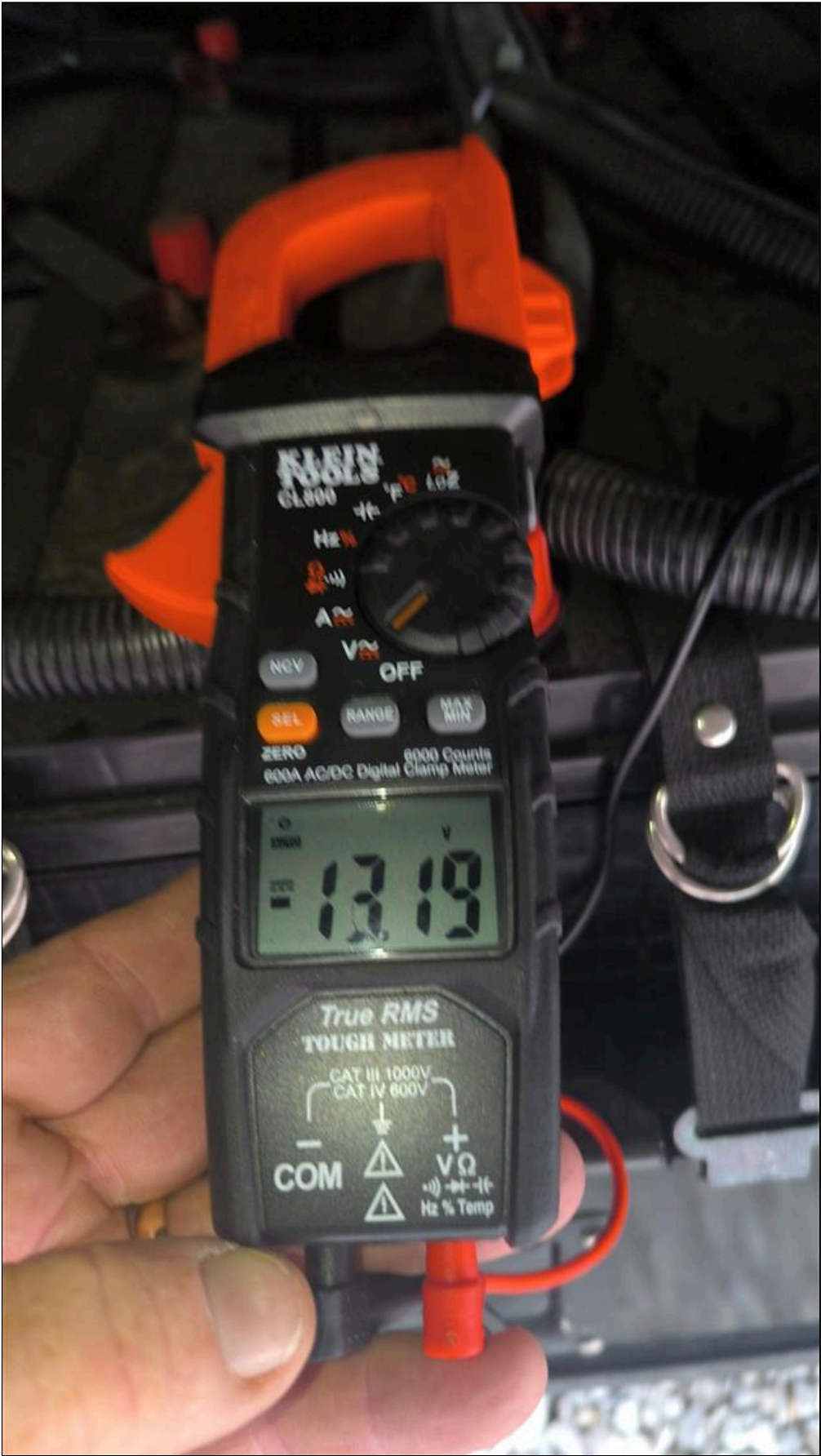
14.3 Hot Skin Test - Was any Frame and Running Gear Voltage Recorded
