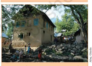
In villages of Kashmir, houses are made from stones cut and kept one on top of the other and coated with mud. Wood is also used. The houses have sloping roofs.
