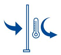
Utilising an invisible coating, low-e, or low emissivity, glass works by reflecting heat back inside your home. It also allows more solar radiation through than standard glass, leading to an increase in heat through passive solar heat gain. This ensures for a warmer home in the winter time, but it can lead to homes becoming too hot during the hotter months.
