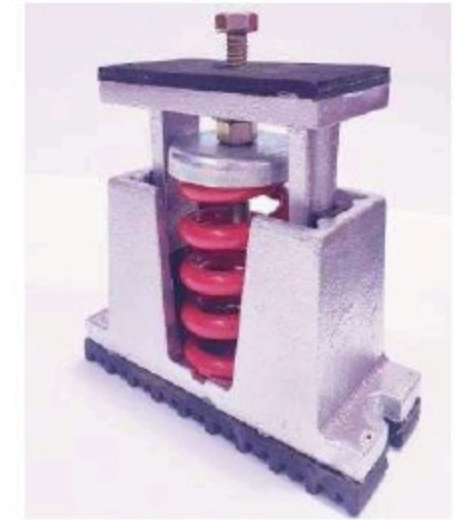
CASED SPRING MOUNT 50 MM DEF. MODEL HSML 25 KG TO 4000 KG
