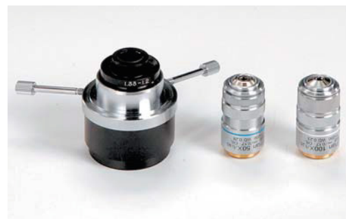
ARKFIELD CONDENSER AND OBJECTIVES WITH IRIS DIAPHRAGM
