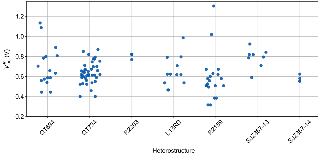
Figure 3.41: Comparison of the barrier-barrier pinch-off voltages V_{po}^B for different heterostructures. The random horizontal spread ensures visibility and has no physical meaning.
