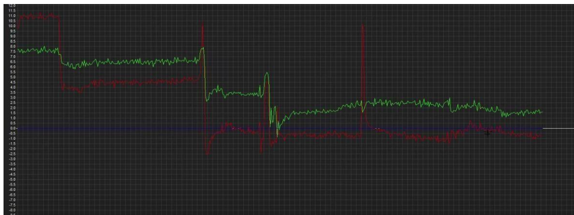
4.18 Degrees v Time Results of the Complementary Filter applied on IMU readings. Pitch (Green) and Roll (Red). Complementary coefficient – 0.02
