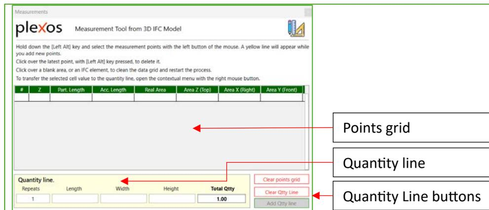
Figure 20 Digital Measurement Tool
