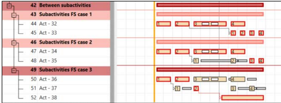
Figure 13 Criticality between sub-activities (Gantt Chart)
