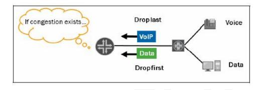
You can associate a loss priority with a packet to tell the system which priority it should give ti dropping this packet during congestion. If you choose to configure RED, you can choose different drop probabilities for traffic with different loss priorities.
