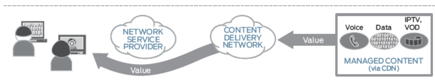
Figure 1.8. High level view of CDN delivery model
