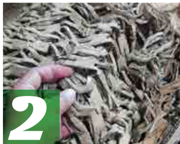
2 SHREDDING OF THE LEATHER SCRAPS INTO FIBERS
