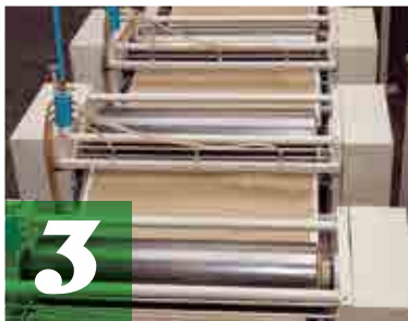
3 BONDING THE SHREDS WITH NATURAL RUBBER
