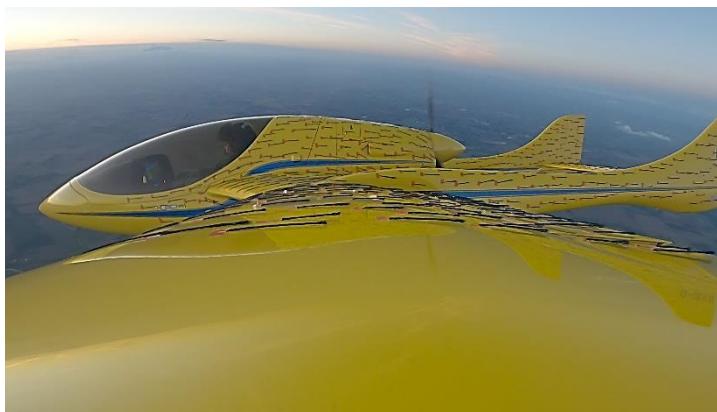
Laminar flow over the aircraft in straight and level flight indicated by aligned tufts.
