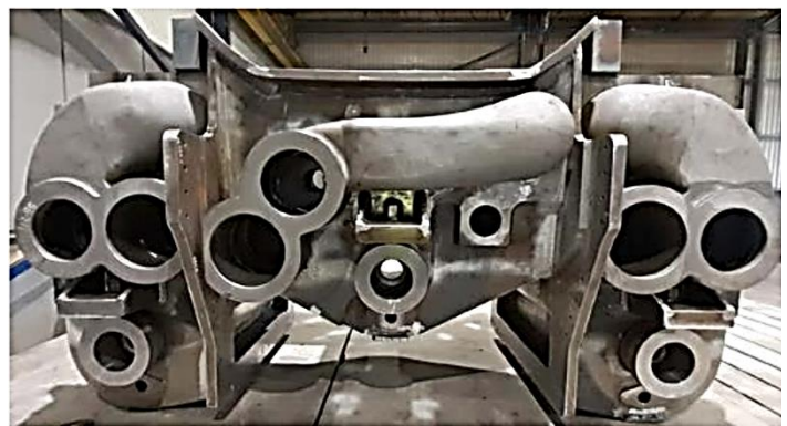
Rear View Of Cylinder Monobloc.
