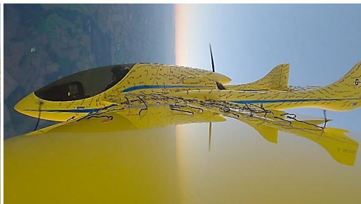
Separated air flow over the aircraft at entry to spin as indicated by disturbed tufts.
