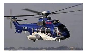
The Super Puma was upgraded when Eurocopter became Airbus. It became the Airbus EC225 Super Puma. All of these 19-seat aircraft were faster with longer range. The EC225 could fly for about 4½ hours.
