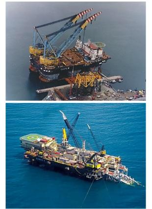
Crane Barges: In structural installations there have to be some very large crane barges.
