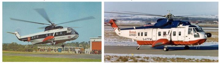
In Penzance Cornwall, BEA, (now British Airways) were operating Sikorsky S-61N helicopters. These offered a scheduled service between Penzance and the Isles of Scilly. Depending on the temperature and weather conditions, these could carry up to 22 passengers at a time.
