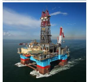
This is a more "state of the art rig". It is a modern semi-submersible drilling rig, with two pontoons located under the water line. It is fully motorised, and it can move itself around the world at great expense.
