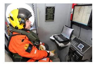
Inside the S-92, the winch operator had his own station in the front of the cabin. The winch operator controlled the radios, the computer system charts, including ordnance survey maps and multiple charts of the area. The information brought up on the winch operator's screen could be superimposed on one of the screens in the cockpit.
