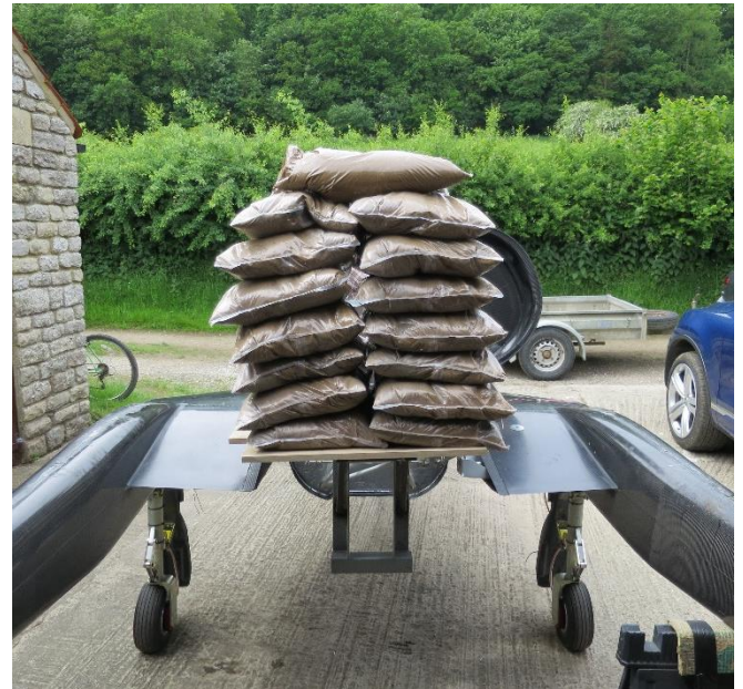
Engine Frame Proof Loading = 827 lb (375 kg)
