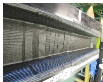
Spar Moulds and a Spar being layed Up.
