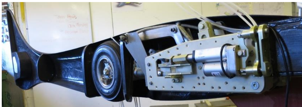
Main Gear Retracted Into Half Boom To Show Complexity Of Fit
