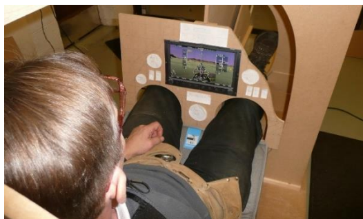
Checking Instrument Ergonomics
