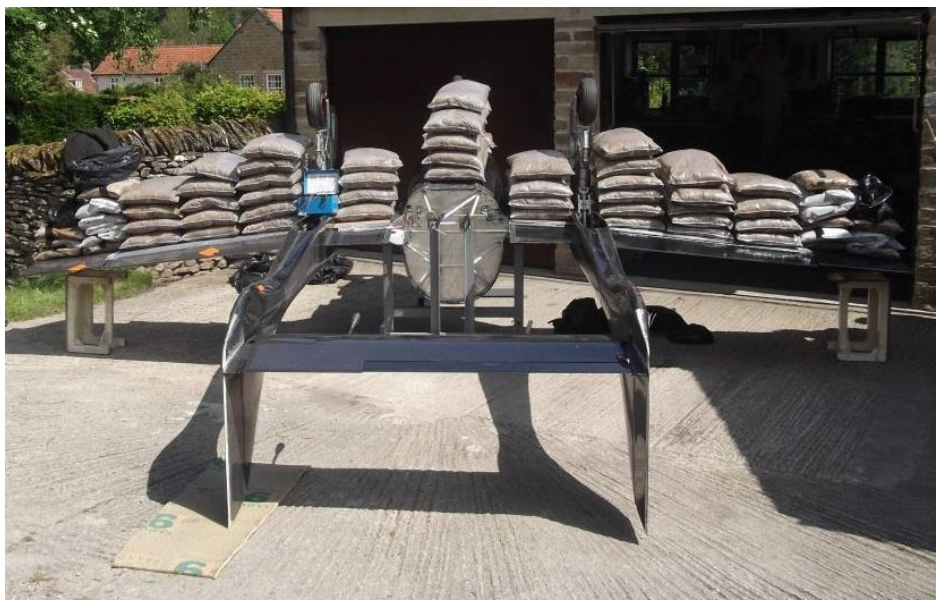
Wing Proof Loading = 3890 lbs (1764 Kg) Wing Tip Deflection 60mm
