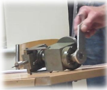
Tightening up the R8 horizontal collet
