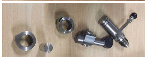
Assembly showing head and valves (including holding mandrel)
