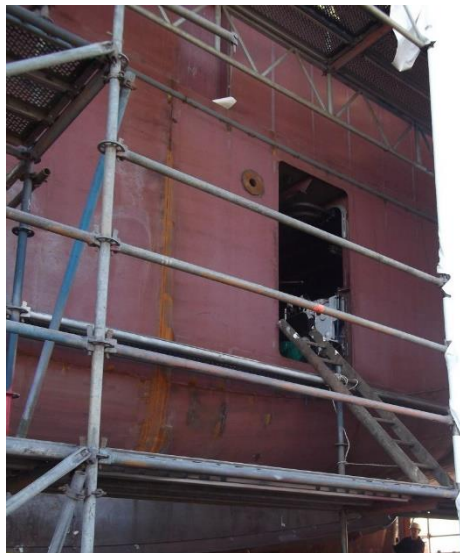
Access cut in hull for auxiliary engine installation
