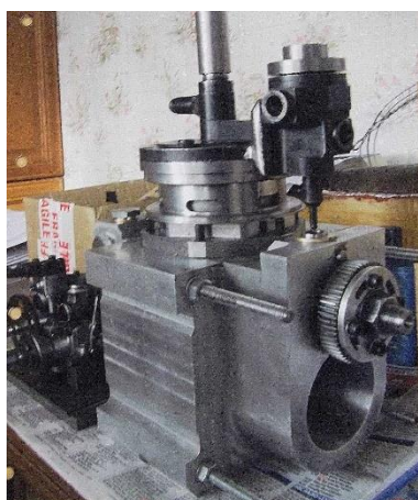
Assembly showing head and valves (including holding mandrel)
