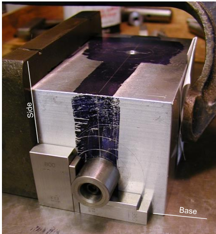
Attaching A Toolmakers Button Using Slip Gauges
