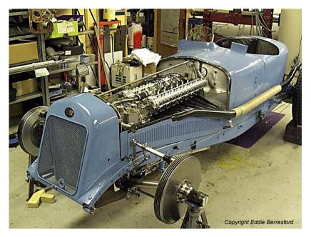
One problem with the *Delage* is that the engine is offset from the centreline of the car. It is a 100mm offset on the full-size car and 40mm in the model. The offset is to the left hand-side of the car to give more room for the driver on the right-hand side.
