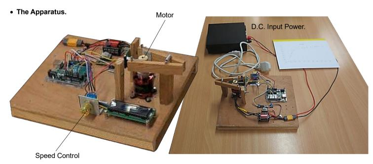
David has built the monitoring apparatus here, which is a test bed. He can generate a pulse, with a modulated signal to go to the speed controller, and then he can measure the speed of the motor.
