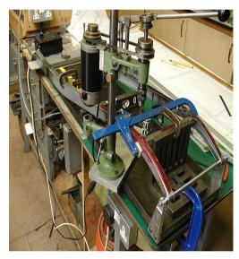
Here Mike has set up a *George Thomas* drilling machine, so he can start to drill the rivet holes for riveting in the chassis cross members.
