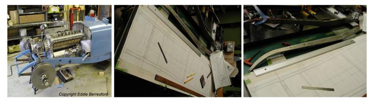
The first thing that was done was to produce a drawing of the chassis to the correct scale. Mike did have enough information to produce the profile of the chassis, and the position of all the cross-members. The profile of the chassis can be seen at the back of the drawing board. This was sawn out of <sup>3</sup>/<sub>4</sub>" aluminium plate, reducing the depth of the shape by twice the thickness of the 2mm steel sheet to be wrapped around it.
