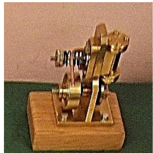
'Rory's Rocket' Double Oscillating Engine. Freelance design by the builder. Builder: David Proctor
