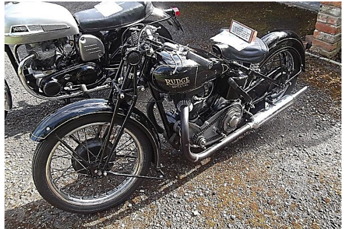
1937 Rudge 500** Bought at Auction. Found a well worn engine and a broken frame. Restored by Jonathan Milner.
