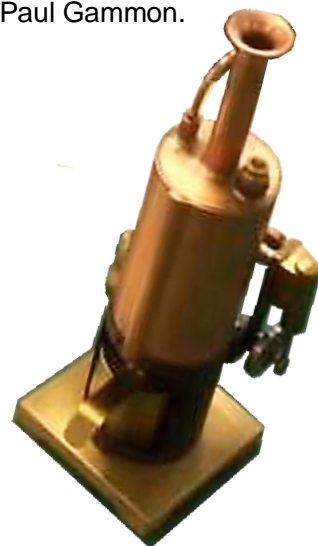
Oscillating Engine. Built to 'Tubal Cain' Design Builder: Dave Dobson.
