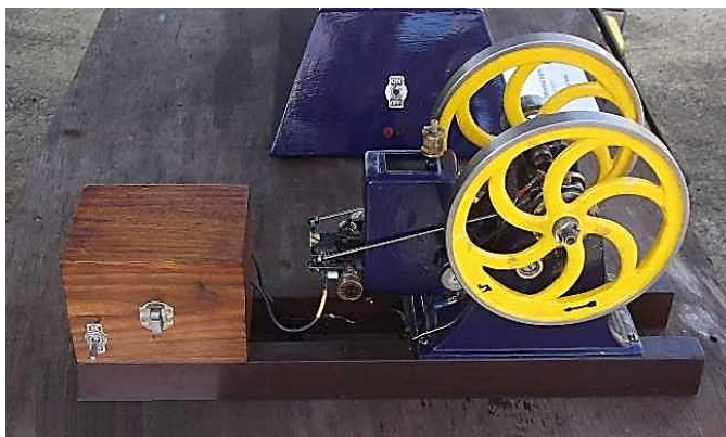
Above: Atkinson Cycle Engine ~ Runs On Petrol. Built by Mel Doran.
