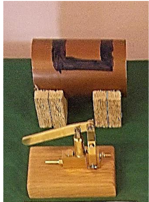
Boiler Feed Pump and Boiler (Work In Progress). To the Martin Gearing Design as published in The Model Engineer 4576-4615 Builder: David Proctor
