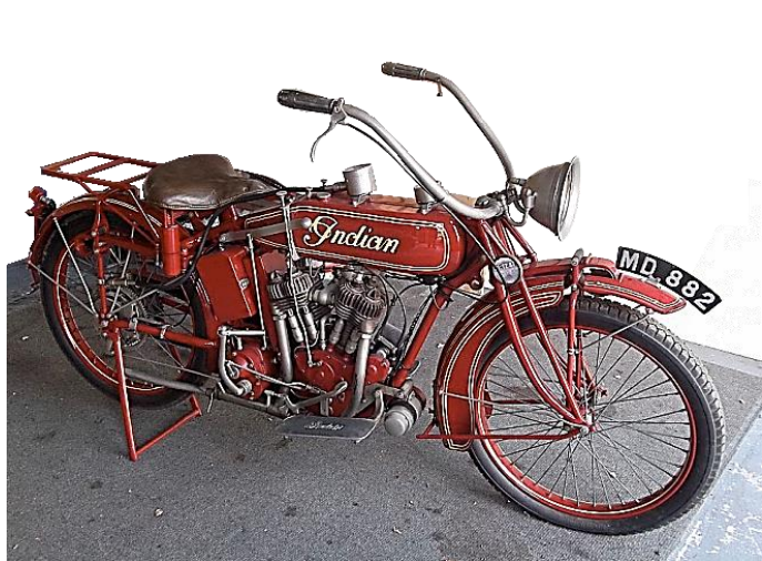
1919 Indian Powerplus 1000cc V twin. Constructed from a pile of spares bought by Mike Sayers and his Dad.
