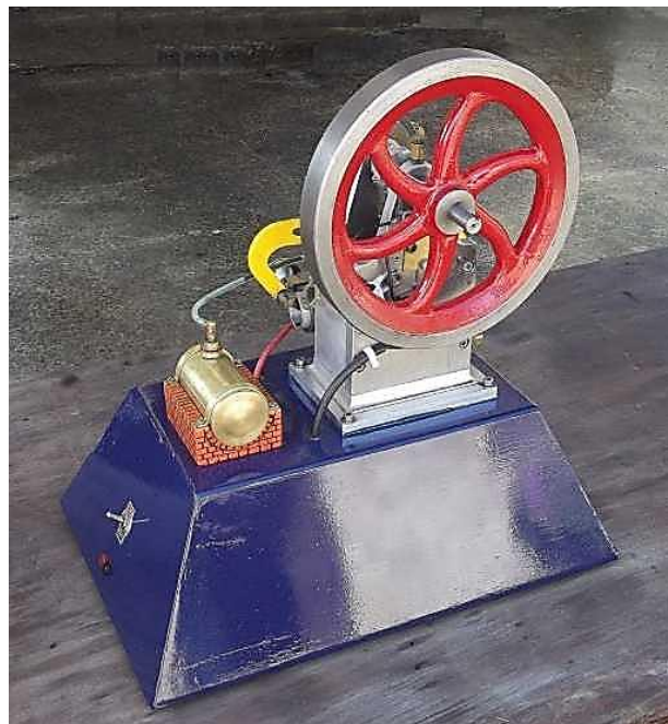
Atkinson Differential Engine ~ Runs On Petrol. Built by Mel Doran.
