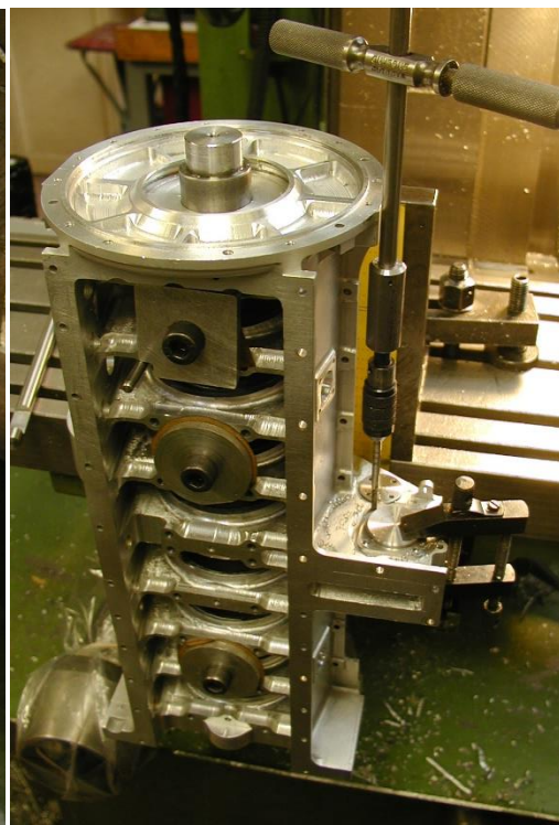
Photo 6: Tapping 6BA Holes For The Large Bearing Boss. A Near Miss In This Case!
