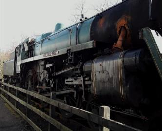
Next to the "Wheel Drop" was 75029 "Green Knight" a Standard Class 4 4-6-0 which is ready for restoration. The fittings have been removed ready for a boiler lift.
