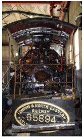
The boiler was overhauled at Crewe, and immediately a boiler is hydraulically tested, its ticket starts running for 10 years from that point. The locomotive is to have the boiler retested hydraulically to restart the ticket. With its overhaul completed at the Grosmont MPD it will then run on the NYMR. There had been problems aligning the smoke box, and a new smoke box has had to be fitted in. The smoke box on this engine is not round.
