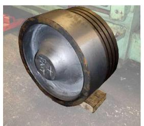
We also saw the axle boxes for the 'Sir Nigel Gresley' bogies. The boxes have already been "white metalled", and are awaiting measurements so that they can be finally machined off
