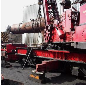
The "Wheel Drop" facility was next on the tour. This is a great asset for the MPD, because instead of having to lift the engine to remove wheel sets, the wheel sets can be dropped to reach the springs. Here we see a British Railways Standard Class 4MT 2-6-0 in the facility.
