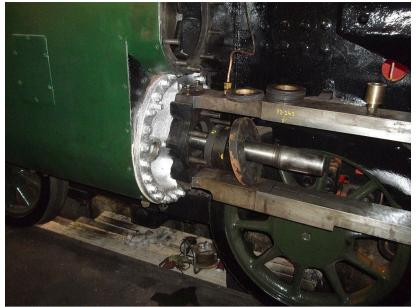
We then looked at the work on S15. Some of the rods were on, and the crosshead is being machined elsewhere and will be "white metalled". For S15, some parts have been machined at the MPD and some have been machined elsewhere.
