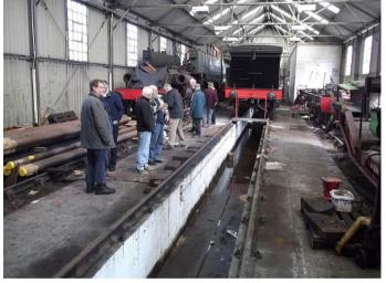
In front of No. 5 was BR Standard 4 Tank 80135 2-6-4T, which also belongs to NYMR. This engine is currently in the shed while it awaits boiler repair.
