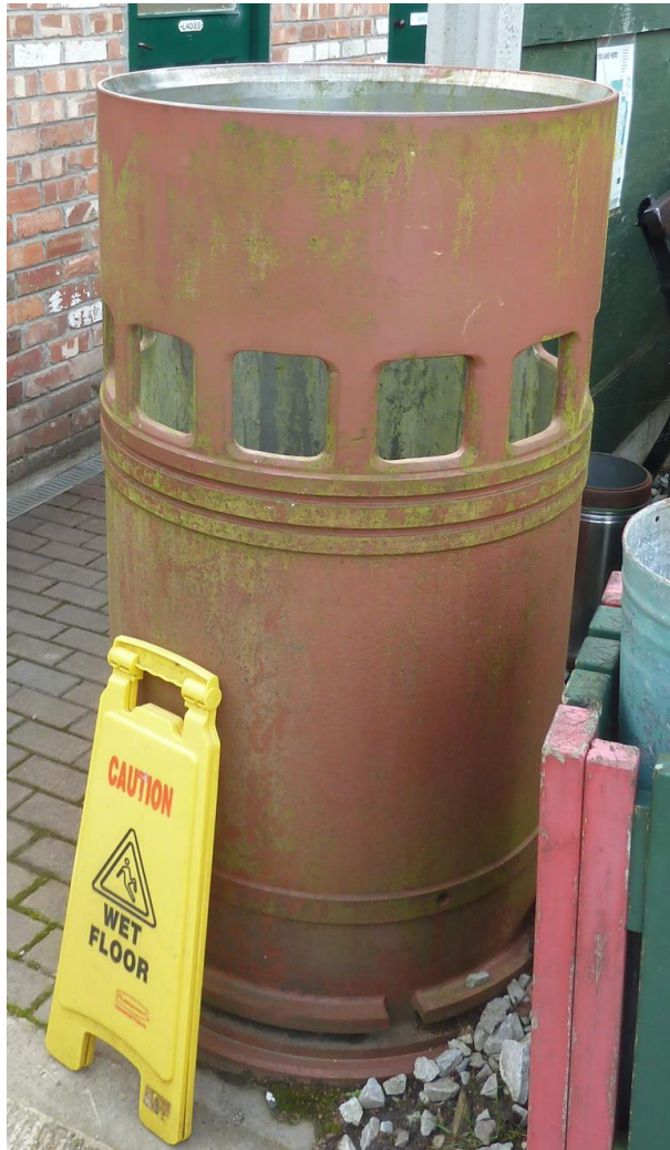
Lower cylinder liner – Photo: David Proctor
