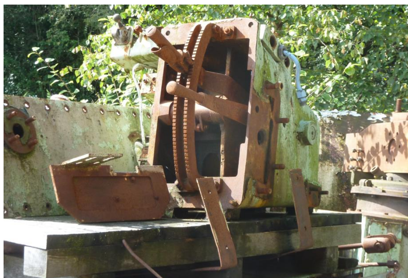
Doxford control stand – minus fuel pressure wheel! Photo: David Proctor
