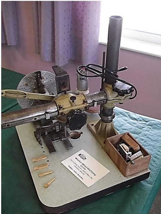
Wooden Wheel Machining Centre for making spokes and felloes for wooden wheels. Peter Bramley
