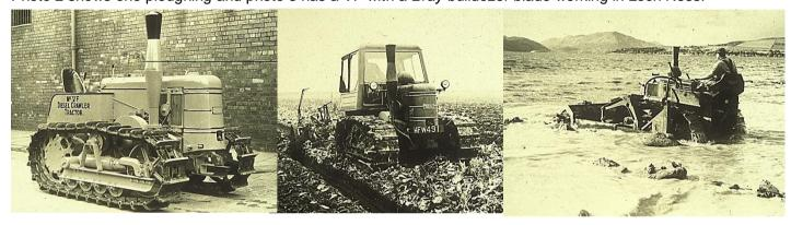
The next tractor to be developed was the Series 3. It had slightly different bodywork, bigger wheels and a bigger engine. A lot were exported to Canada and some were sent back for improvement and this developed into the 3A. The second photo shows the prototype 3A. The flyheel and the engine were more or less the same size as the Series 3 with a 6" bore single cylinder.
