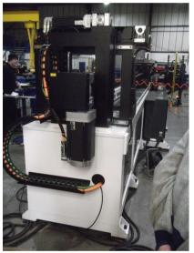
We were shown a three-axis machine which allows a tube to be first bent one way and then the other. The more axes that are added, the more complicated the control and the greater the expense. The 3-axis machine is fairly typical. There are a great many safety features on the machine.
