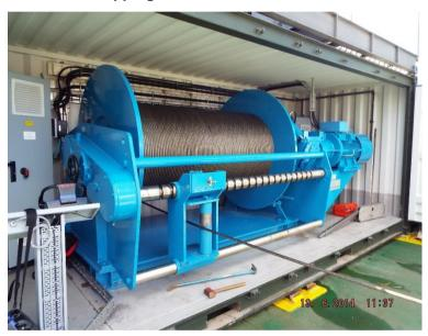
This is a 15 tonnes winch that went to Sweden. This was supplied to the Swedish Polar Exploration Society. They requisition an ice breaking tug each year for a three-month scientific exploration. There is 6000 metres of cable on the winch, and at the end is a subsea core sampling device. This is launched into the sea bed to a depth of 3 metres. The core sample is analysed on the vessel.
