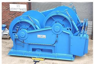
Instead of having one drum doing two jobs, here each drum does its own job. One drum is for towing and the other drum for anchor handling. This is what is known as a 'waterfall configuration'.
