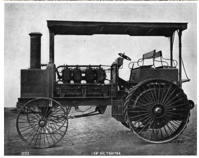
The four cylinder 60 hp 'Oil Tractor' is shown on the left.
