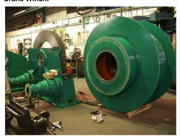
This was manufactured before NSW had the new fabrication shop on site. This photo shows the assembly of a crane winch. There are two epicyclic gear boxes. There are also big output pinions. The ring gear is bolted to the drum. It is direct drive "power in power out". Theses winches are rated at 40 tonnes. They went on a crane barge for a Dutch company who are involved with industrial size automatic lock gates.
