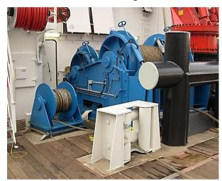
This is mounted on a tug. The 50 tonnes rating is based on the torque applied through the outer diameter of the cable. On core, the rating is 80 tonnes. This winch is for towing duties and anchor handling.
