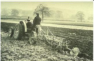
Besides towing and being used 'on the belt', the tractors were used for ploughing. Here is a preproduction Model 'M'.
