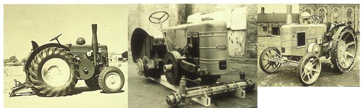
The following photograph shows the VFA caterpillar tractor which was developed from the 3A. With regard to wheeled tractors, Marshalls decided that the future lay with multi-cylindered engines and built two four-cylinder engined MP4s (second photo).
