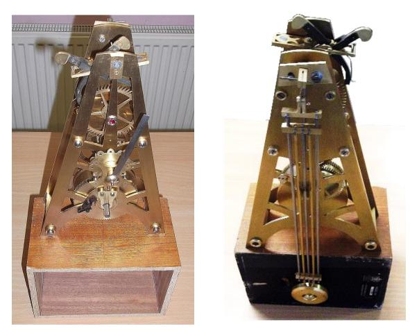
John said that we have seen this before. It is a freelance timepiece based on Harrison's work. The idea behind it was to make as many parts that can move around for interest's sake. However, that coupled with the scaling down from Harrison's work has created a lot of problems, which may turn out to be insurmountable.
