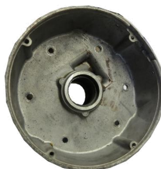
Front Of Crankcase Showing Bearing B1 Bush
