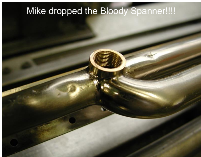
Final intended operation tapping the pressure relief valve boss to remove plating.
