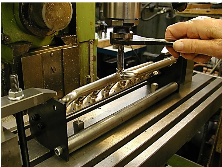
Final intended operation tapping the pressure relief valve boss to remove plating.
