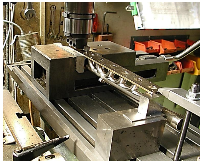
Fly cutting the damaged mounting flange.
