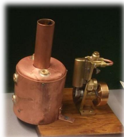
Boiler For Model Windermere Steam Boat ~ John Heeley
