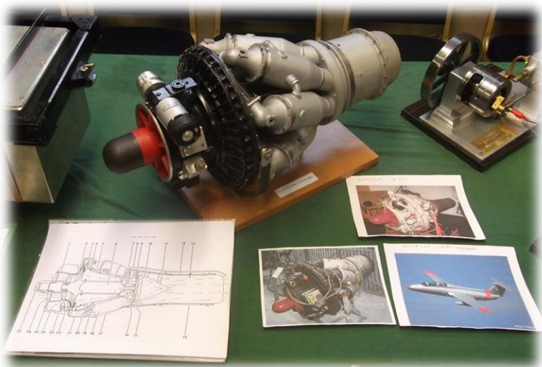
1/4 Scale Czech Motorlet M-701 Turbojet For The L-29 Trainer Aircraft ~ John Heeley
