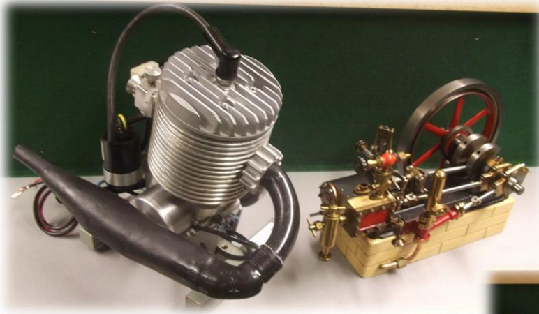
32cc 2 Stroke Engine John Heeley
