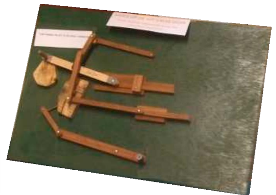
'Chelmsford' Steam Car and a mockup of the 'Joy' Valve Gear for the car ~ Peter Bramley
