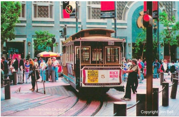
The single ended cable cars are turned manually on turntables at the termini by the driver and conductor.
