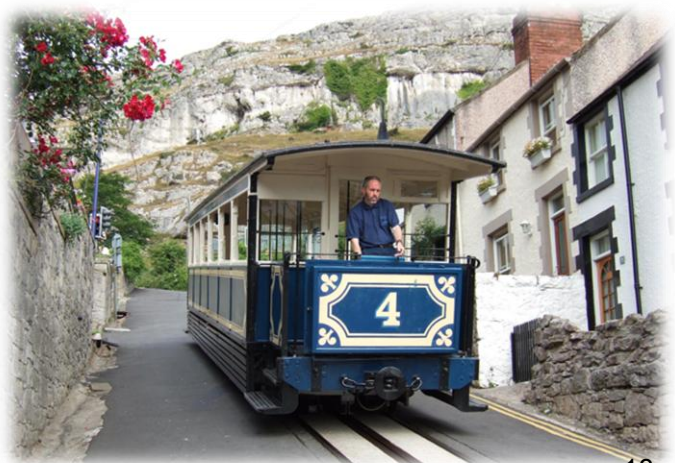
The Great Orme Tramway is on the right. The slot between the rails can be seen.
