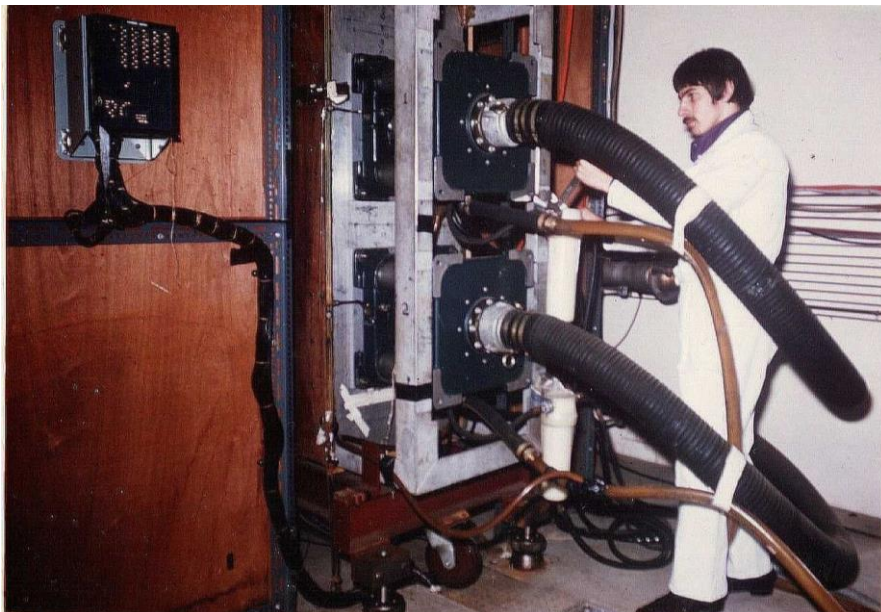
Working on the blowers in the Noise Room
