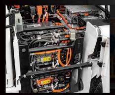
High-efficiency power system and high-performance lithium iron phosphate battery: the lithium battery is installed horizontally. With the standard water cooling system **(For 35-50t)**, the battery can last for a long time.
