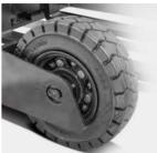
The front wheels are equipped with deep groove rubber tires, with large ground clearance, wear resistance and durability, and good shock absorption effect.
