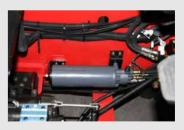
The seat sensor system incorporates lifting/tilting and traveling locking function.When the operator leaves the seat, the system automatically locks lifting/tilting and disables traveling to ensure safety.
