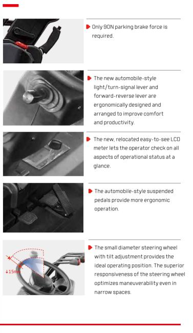
In developing the new XF 8-12t series, comfort and easy operation is always considered, for example, inproved vibrating levels, compound engine damper and full floationg seat and cabin are applied.
