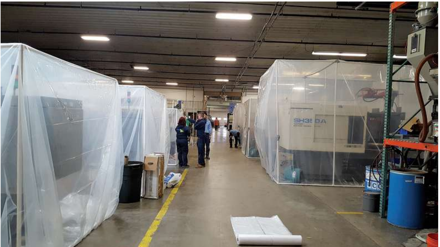
IVP Plastics employees set up a makeshift triage unit for 17 injection molding machines that took a soaking after the roof collapsed and brought down a piping system connected to a water tower.
