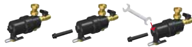
Closing the shut-off valve. Removing the magnet (turn it 90 clockwise). Unscrew the filter chamber
