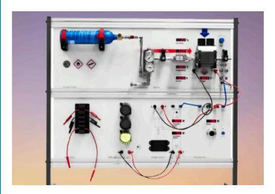
Fuel Cell Training System is a standalone, modular educational platform designed to help students and researchers understand the practical workings of hydrogen fuel cell technology. The system demonstrates how electrical power is generated using dry hydrogen, regulated, stored, and supplied to real-world DC and AC loads—enabling a complete learning experience in sustainable energy systems.
