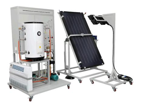
The Solar Thermal Flat Plate Collector (FPC) Trainer is designed to demonstrate the fundamentals of solar water heating using non-concentrating solar thermal technology. It enables students to analyze thermal performance under varying conditions and understand solar heat transfer principles.
