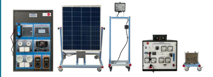
The Solar PV Trainer provides practical exposure to photovoltaic power generation, enabling learners to explore solar energy harvesting, electrical characteristics of PV modules, and performance under various conditions.
