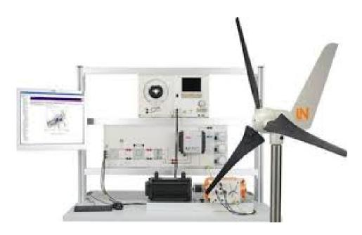
Designed to simulate wind energy generation, this trainer includes a lab-scale wind turbine setup for studying turbine characteristics, power output, and aerodynamic effects under controlled wind conditions.
