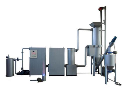
This trainer demonstrates biomass gasification, converting solid biomass into producer gas using a down-draft gasifier. It aids in understanding combustion zones, syngas generation, and renewable fuel applications.
