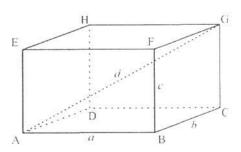
In three dimensions, the magnitude of the vector  $\begin{bmatrix} a \\ b \end{bmatrix}$  is  $\sqrt{a^2 + b^2 + c^2}$
