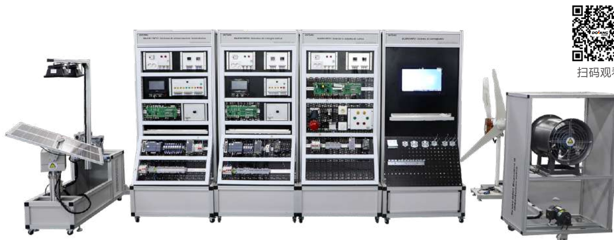
DLXNY-WP01型风光互补发电实训系统 Wind Solar Complementary Power Generation Training System
