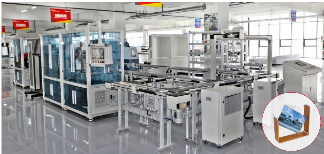
DLIM-3119 智能制造礼品相框生产系统 Intelligent Manufacturing Gift Frame Production System
