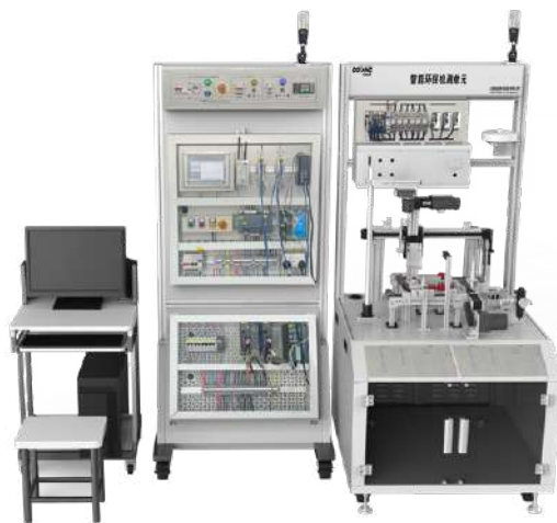
DLIOT-231 工业网络编程与调试应用系统 Industrial Network Programming and Debugging Application System
